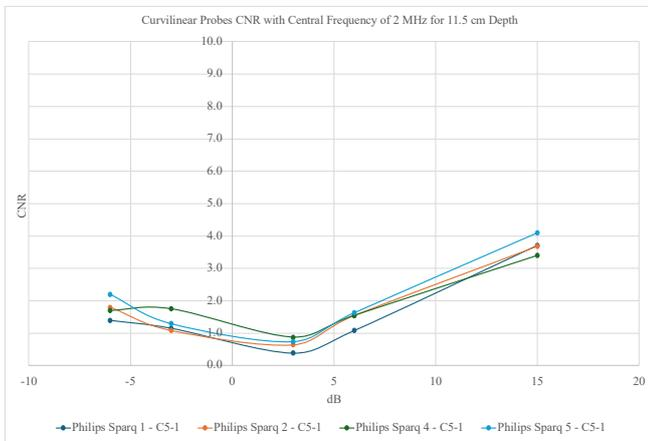
Fig. 8. A graph which represents the CNR of four curvilinear probes
