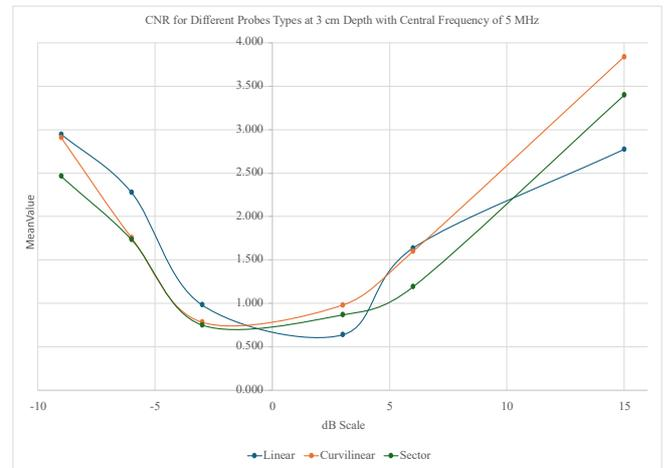
Fig. 21. Mean CNR against dB scale for different probes with a common frequency of 5 MHz and at a depth of 3 cm
