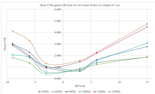
Fig. 14. Mean CNR against dB scale for all linear probes at a depth of 3 cm
