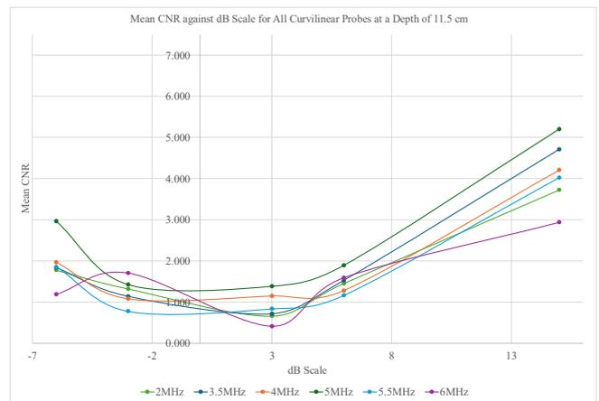
Fig. 17. Mean CNR against dB scale for all curvilinear probes at a depth of 11.5 cm
