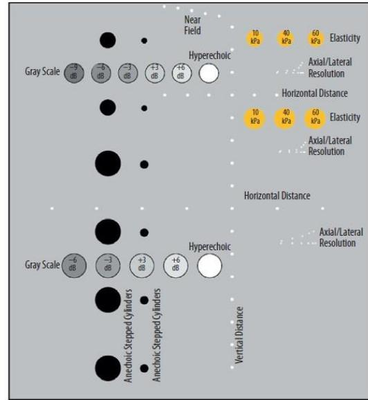
Fig. 4. A schematic for the phantom model CIRS 040GSE, Fabiszewska et al. (2017)
