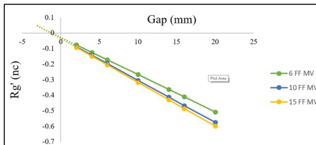
Figure 4: graphical representation of the variation of DLG versus 6 MV, 10 MV and 15 MV photon beam energy.
