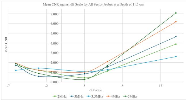
Fig. 18. Mean CNR against dB scale for all sector probes at a depth of 11.5 cm
