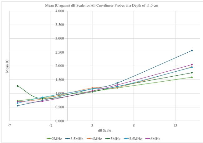
Fig. 12. Mean IC against dB scale for all curvilinear probes at a depth of 11.5 cm
