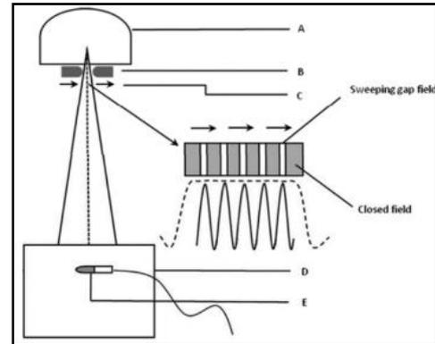
Figure 1: Schematic diagram of DLG measurement using ionization chamber.
