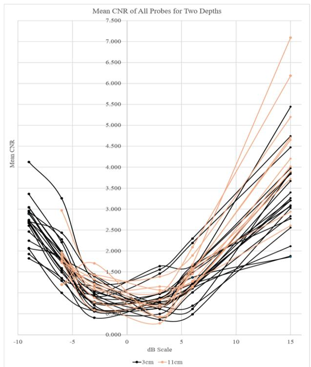
Fig. 24. Mean CNR against dB scale for all probes at two different depths
