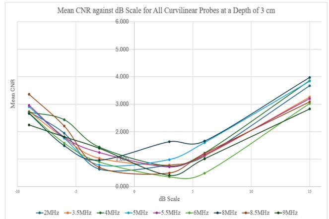
Fig. 15. Mean CNR against dB scale for all curvilinear probes at a depth of 3 cm
