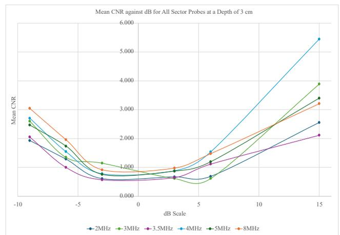
Fig. 16. Mean CNR against dB scale for all sector probes at a depth of 3 cm
