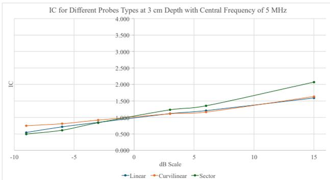
Fig. 19. Mean IC against dB scale for different probes with a common frequency of 5 MHz and at a depth of 3 cm
