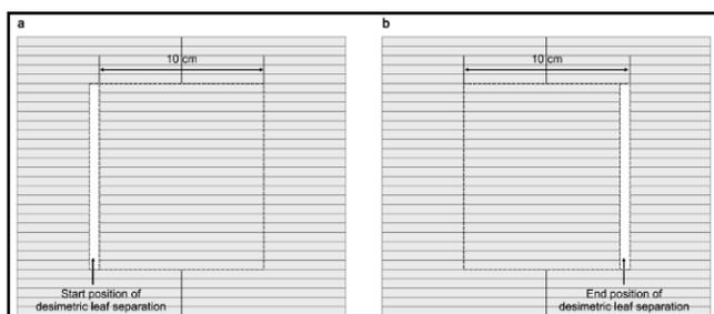
Figure 2: Start (a) and end (b) position of the 10 mm sliding slit movement for dosimetric leaf separation file.
