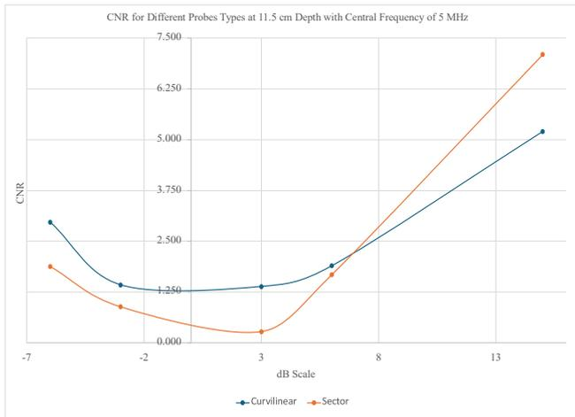
Fig. 22. Mean CNR against dB scale for different probes with a common frequency of 5 MHz and at a depth of 11.5 cm
